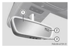
To receive a correct display in rear-view mirror (1), the compass must be calibrated and the magnetic field zone set.
