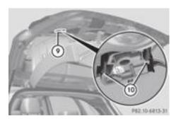
► Remove bulb holder ③ using both sides of lever ⑩.
