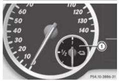
Condition of charge display ① shows the condition of charge of the high-voltage battery. The charge values are shown as a percentage in the COMAND display (see the separate operating instructions).
