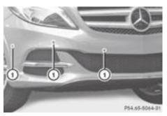
① Example: sensors in the front bumper, right-hand side
