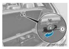
▶ Fold out hook ③ on the underside of the cargo compartment floor.
