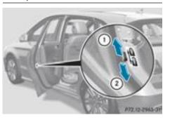
You secure each door individually with the child-proof locks on the rear doors. A door secured with a child-proof lock cannot be opened from inside the vehicle. When the vehicle is unlocked, the door can be opened from the outside.
