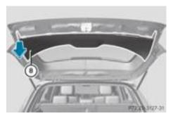
▶ Unclip part of trim (a) from the assembly using a sudden, sharp movement, until bulb holder (b) is accessible.
