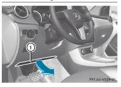
Driver's knee bag (1) deploys under the steering column. The driver's knee bag is triggered together with the front air bag.
