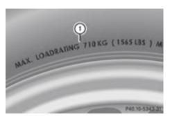
Maximum tire load ① is the maximum permissible weight for which the tire is approved.
