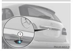
Rear view camera ① is in the handle on the tailgate.
