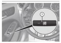
▶ To activate/deactivate: press button (1). If indicator lamp is lit, operation of the rear side windows is disabled. Operation is only possible using the switches in the driver's door. If the indicator lamp is off, operation is possible using the switches in the rear compartment.
