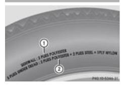
This information describes the type of tire cord and the number of layers in sidewall ① and under tire tread ②.
