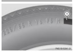
In addition to the load bearing index, load index 1 may be imprinted after the letters that identify speed index 6 on the sidewall of the tire ( $\triangleright$  page 293).
