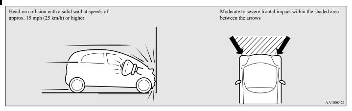
The front airbags are designed to deploy when the vehicle suffers a moderate to severe frontal impact. A typical condition is shown in the illustration to the left.
