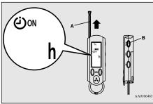
2. To turn the MiEV Remote off, press the power/communication switch (B) for 3 seconds or more and store the antenna (A).
