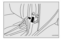
This placard shows the maximum number of occupants permitted to ride in your vehicle as well as "the combined weight of occupants and cargo" (C), which is called the vehicle capacity weight. This placard also tells you
