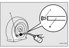
11. Holding the sealant bottle upside-down, squeeze it again and again to inject all of the sealant into the tire.
