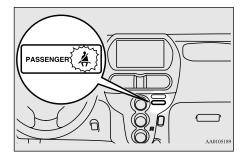
When the electric motor switch is turned to the "ON" position, this indicator normally comes on and goes off a few seconds later. The light comes on when a person sits on the front passenger seat but does not fasten the seat belt.
