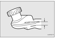
The brake fluid level falls slightly with wear of the brake pads, but this does not indicate any abnormality.
