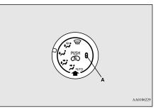
If high cooling performance is desired, or, if the outside air is dusty or contaminated in some way, use the recirculation position. Switch to the outside air position every now and then to keep the windows from fogging up.
