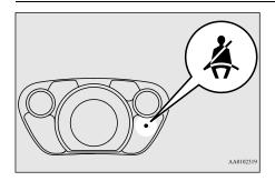
If the electric motor switch is turned to the "ON" position without the driver's seat belt being fastened, a warning light will come on, and a tone will sound for approximately 6 seconds to remind you to fasten your seat belt.
