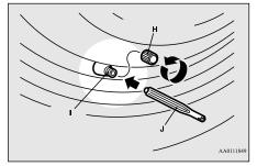
9. Remove the valve insert (K) by turning it counterclockwise using the valve remover (J). Put the removed valve insert in a clean place so it does not get dirty.
