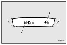
A- Adjust mode B- Adjust level
