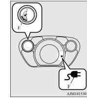
• Turning the electric motor switch to the "ON" position or the "ACC" position will cancel the Charging Timer.
