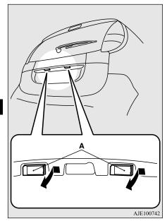
2. Use a flat blade screwdriver into the tab (B) and pry gently to remove the lens.
