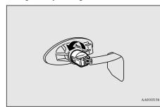
3. Pull the bulb out of the socket.
