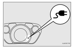
If the charging indicator is not illuminated, charging has not started. Refer to the quick charger user manual.
