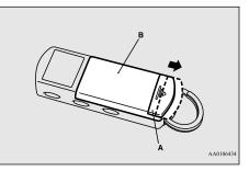
3. By moving the battery cover (B) in the arrow direction, tabs (C) on the battery cover will come out and the battery cover can be removed.
