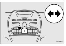
If you press the flasher switch, the front and rear turn signals will flash intermittently, and so will the hazard warning lights. This is an emergency warning system and should not be used when the vehicle is in motion, except for emergencies.
