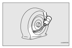
13. Pull out the compressor hose (N) from the side of the tire compressor, and then securely attach the hose to the tire valve (I).
