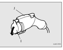
9. Connect the regular charge connector until a click is heard without pressing the button (K).
