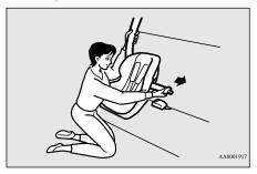
3. To activate the ALR child restraint installation function, slowly pull the shoulder part of the belt all the way out of the retractor until it stops. Then let the belt feed back into the retractor.
