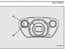
When the electric motor switch is in the "ON" position and the remaining bar of the energy level gauge shows 2 bars or less, the warning indicator (A) and the charging bars (B) flash as follows:
