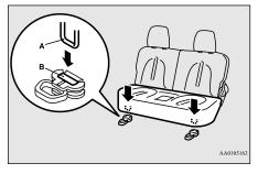
5. After installing the seat cushion, shake it lightly to confirm that it is properly fixed in position.
