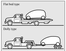
Towing with rear wheels off the ground
