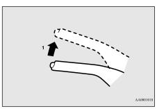
Pull the lever up without pushing the button at the end of hand grip.
