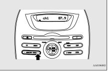
3. To recall a frequency that has been saved in memory, press the MEMORY button briefly for no longer than about 1 second.
