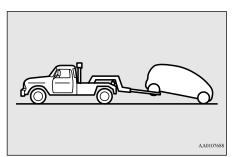
Place the selector lever in the "N" (NEU-TRAL) position. Turn the electric motor switch to the "ACC" position and secure the steering wheel in a straight-ahead position with a rope or tie-down strap. Never place the electric motor switch in the "LOCK" or "ON" position when towing.
