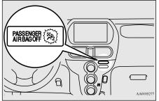
The indicator normally comes on when the electric motor switch is turned to the "ON" position and goes out a few seconds later. In the following situations, the indicator will stay on to show that the passenger's front airbag is not operational.
