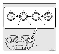
1. Push the reset button (D) to view the driving distance or number of months remaining until the next periodic inspection.
